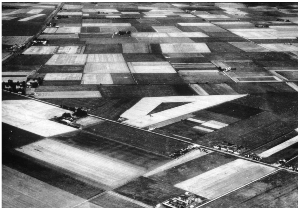
Category 1: Flat grassland, parkland or bare soil, without hedges and only a few isolated obstructions.
