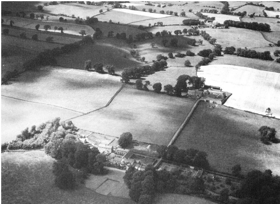
Category 3: Farmland with high boundary hedges, occasional small farm structures, houses and trees etc.
