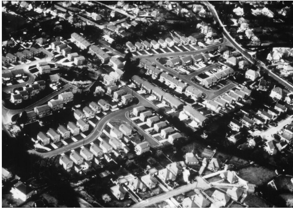
Category 4: Woodland or low rise urban/suburban areas (e.g. domestic housing) with a plan area density of up to about 20%.
